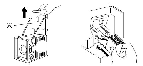
16. Remove the green plastic clip [A] from the staple cartridge, and install the cartridge in the stapler.
