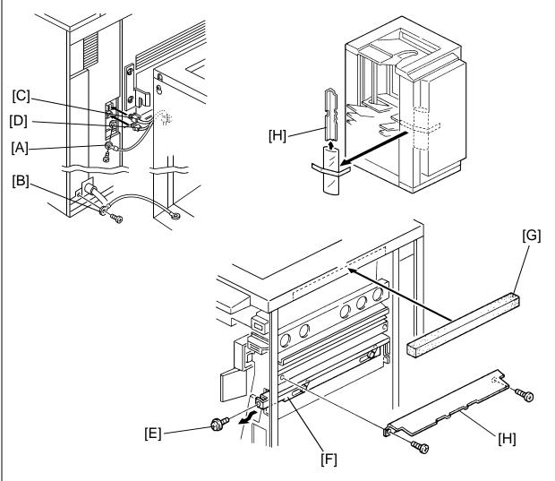
7. Secure the protective earth wire [A]\* (1 screw with spring washer) and the wire [B] (1 screw with spring washer).
